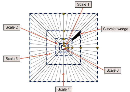
Fig. 1. Default curvelet tiling. 5-scale decomposition is shown. Each scale is divided into  $16 \times 2^{\lceil (j-1)/2 \rceil}$  wedges, where  $j$  is the scale number. Scale locations are denoted by yellow markers.
