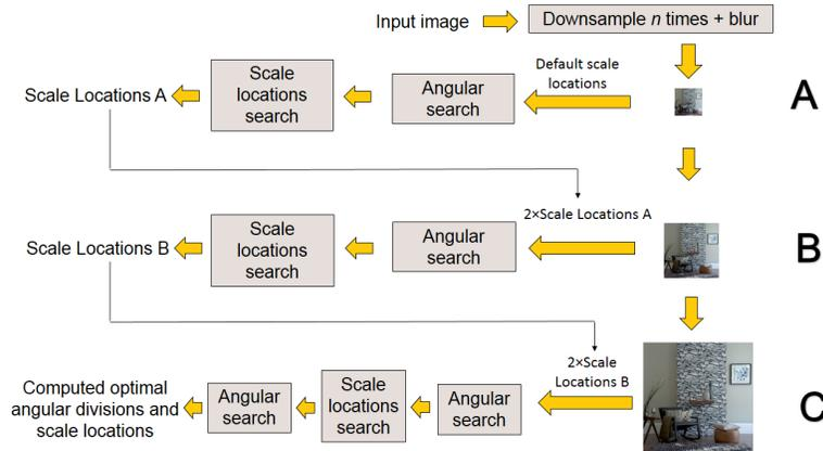
Fig. 2. Flow diagram of the global optimization algorithm.
